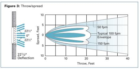
Handbook for a more detailed explanation. Good air distribution design makes use of room surfaces to help keep the supply air outside the occupied zone.
